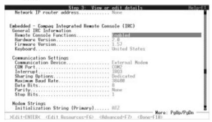
Figure 2-5. Example: Enabling Remote Console Functions
